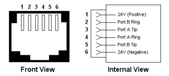
(View of CM connector) CM Port A and B connections. Shown with CM-10 connected.
